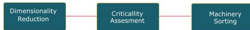
Figure 36 Distributed Algorithm. The approach proposed consists on three methods executed in a distributed manner. The dimensionality is reduced through principal component analysis (First step), the criticality of machine parameters is evaluated through particle swarm optimization (Second Step) and the operation sorting is done through topological sorting.
