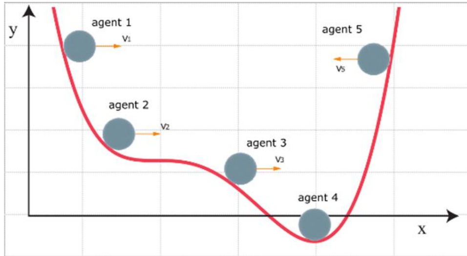
Figure 37 PSO principle. All the elements (agents of the swarm) exchange information while exploring the space to find global minimums of the function to optimize.
