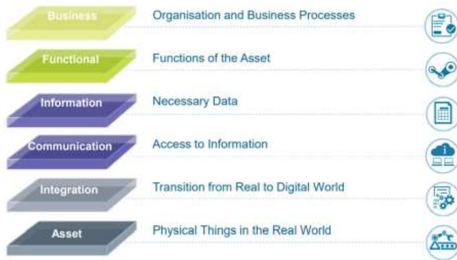
Figure 3 RAMI 4.0 layers on axis 3
